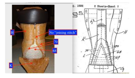
hourglass-shaped stay can save money on materials: The upper leather can be smaller because the two ends don't have to meet precisely at a back Achilles seam. [JA22145 ] 240.]
