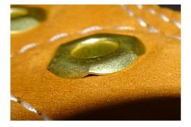
Mr. Whatley explained that the hexagonal eyelets result from crimping the sides of the eyelets to securely affix them to the leather. [JA22146, JA22148–22149 PP 246, 252.] "[T]hese points formed by
