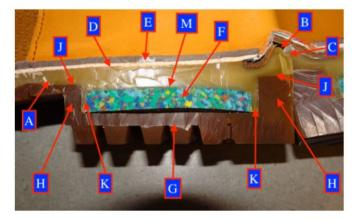
midsole **A** are composed of rubber. [*Id*.] The recess in the heel is filled with a sponge rubber or other soft, springy material **F**. [*Id*.] Using an industry-standard instrument, Mr. Whatley found that the exemplar boot's outsole **G** is about 10-
