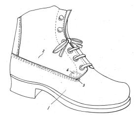
joining the upper and vamp with a notch and a stitch line that curls under the upper in what TBL calls a "U-shape." Mr. Whatley depicted the patent and the exemplar boot side-by-side to show this. [JA22135.] For both boots, the upper and vamp interlock "so that they may be tightly clasped together." [JA22135.]
