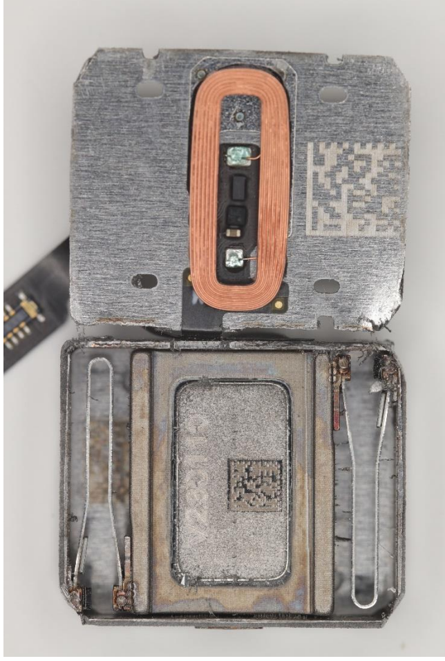
Photograph showing one driving coil (at right) within disassembled Taptic Engine from the iPhone 14, with moveable component in place at left. The moveable component travels up and down from
