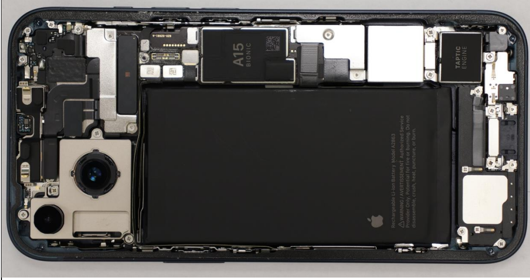
Photograph of iPhone 14 with rear cover removed, with A15 Bionic SoC at center right and Taptic Engine at bottom left.
