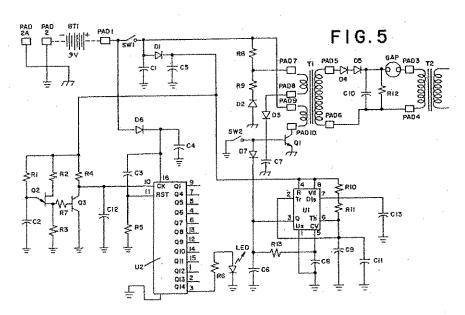
1062-63. The district court identified SW1, referred to by the parties as the "trigger," as a notable component of the circuit and explained that SW1 was a mechanical switch, although the precise type of mechanical switch was not clear from the schematic. <u>Id.</u> at
