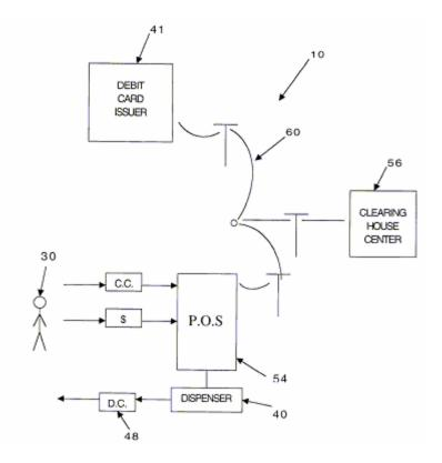
As shown in Figure 1, the card purchaser (30) tenders cash or a credit card to the Point-of-Sale or POS terminal (54). The specification describes the structure of the POS terminal as including "basically a keypad with numbers, letters, names, signs, graphics, with a sliding open side" as well as "necessary input and output hardware such as card charges and card debits 58, computer assembly 60 and associated storage assembly 50." <u>Id.</u> at II. 22-24, II. 36-38.
