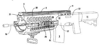
Although the receiver sleeve is "self supported" by its connection to the receiver top, "additional support may be provided by . . . a special yoke about the barrel nut of the firearm." *Id.* col.2 ll.30-36. The yoke, also referred to as a "clamp" at trial, provides this additional support by engaging the firearm's barrel nut. *See id.* col.3 ll.3-9. This engagement occurs roughly in the area denoted by numbers 52 and 63 in the drawing below.
