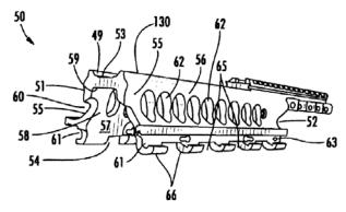
The two support points in the invention (at the receiver sleeve and the barrel nut) permit the upper and bottom handguard pieces to surround the barrel of the gun without touching it. As explained earlier, this design enables a firearm user to operate ancillary devices such as integrated laser devices in complete isolation from the
