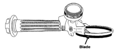
The blade includes an annular groove called a bearing race that enables one or more bearing beads within the housing to engage and support the blade, ensuring that there is no axial movement of the blade during rotation.
