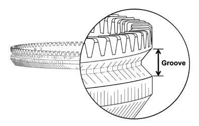
The particular embodiment of patented rotary knife blade disclosed in the specification is depicted with the following cross-sectional view:
