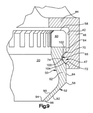
The bearing race is generally indicated by reference numeral 66, and the first and second bearing surfaces are indicated by reference numerals 70 and 72. These bearing surfaces are characterized as being "frustoconical," which the district court defined as "the shape of a portion of an exterior surface of a cone."
