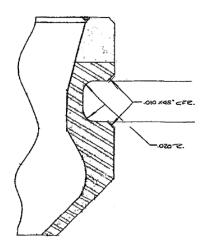
Cross-Appellant Br. 21. As the image reveals, the pre-1998 blade includes two chamfers at the intersections of the bearing race walls and the outer surface of the blade body. According to Bunzl, these chamfers inherently satisfy the frustoconical bearing face limitations because of their shape and their capability "of being in rolling or sliding contact with a support member." Appellant Br. 39.
