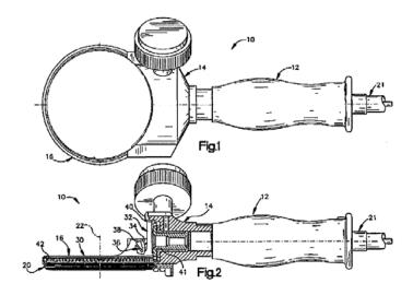
In use, an operator holds the handle and swipes the far end of the annular blade across a piece of meat, for example, to shave off an unwanted layer that moves up through the open center of the annulus and falls off.
